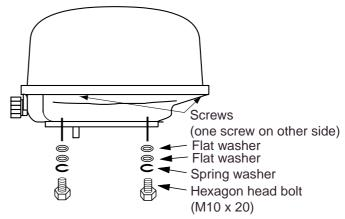
Antenna unit, showing location of mounting hardware
